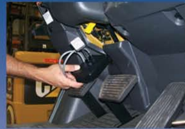
Install KISS-GLWWL under dash OR install KISS-GBWWL on dash
