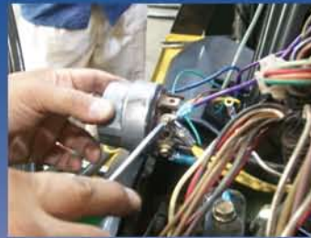
Install relay at ignition switch
